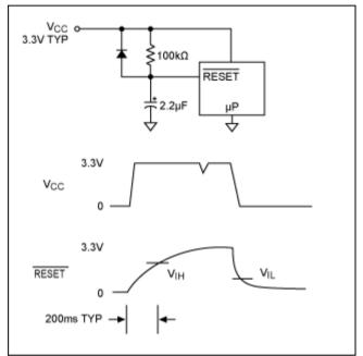
Figure 2. Improved RC delay circuit.
