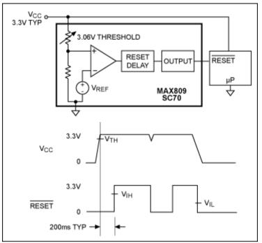
Figure 3. Integrated reset circuit.
