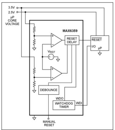
Figure 9. Multiple-supply reset monitoring.
