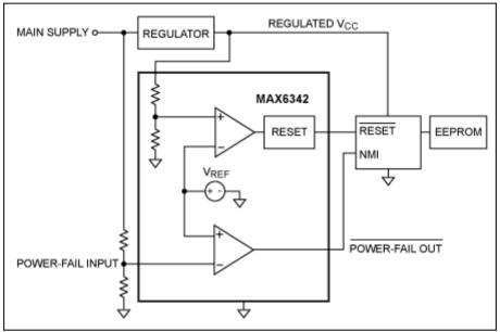
Figure 6. Power-fail/low-battery indicator.
