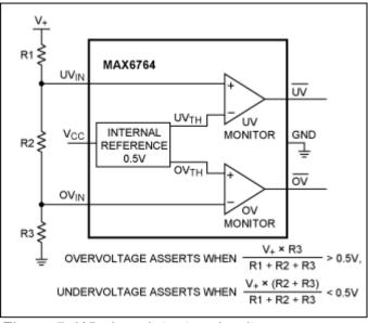
Figure 5. Window detector circuit.
