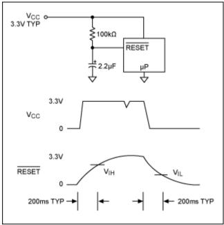
Figure 1. Resistor-capacitor reset delay circuit.
