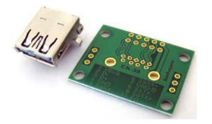
[Product Description] USB3.0 connector (A type: female) is converted to 2.54mm pitch. A connector is included.
