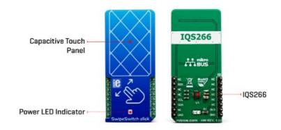
Besides five capacitive touch sensing electrodes, the IQS266 integrates a single proximity channel. This channel can be used to wake up the device from the standby mode when the user approaches the touch panel, ensuring a low overall power consumption that way. CH0 is a dedicated proximity/touch channel and it is treated as a separate channel group in the IQS266 settings. Both proximity and touch thresholds can be defined for this channel.
