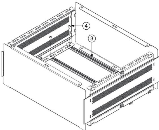
3. Component Mounting Bar assemble use Nut M3 and Screw M3x6
