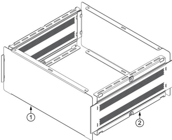
2. Complete Side Frames and Front Rear Panel assembled.
