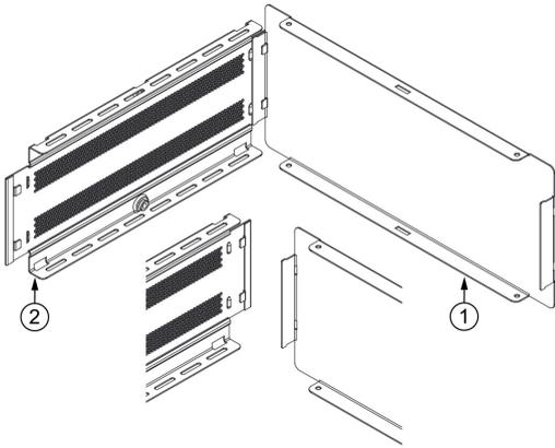
1. Assemble Side Frame to Front Rear Panel.
