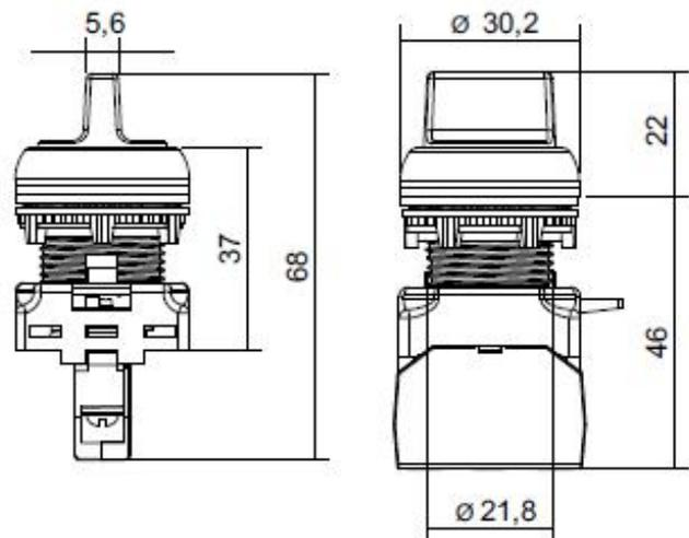
Illuminated 3 position selector switch heads for use with the RS pro modular plastic push button series. Robust design available in Green and Red with modern silver coloured bezel. Simple installation via standard lock nut.
