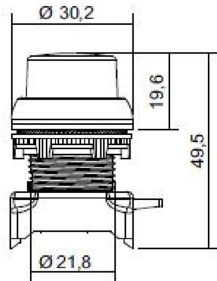
Non-illuminated extended push button heads for use with the RS pro modular plastic push button series. Robust design in a variety of colours with modern silver coloured bezel. Simple installation via standard lock nut.
