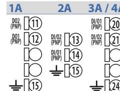
Digital output PNP (including SSR) for command or alarm.
