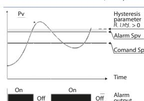
Lower deviation alarm value of alarm setpoint less than "0" and hysteresis value greater than "0" (Par.128  $R_{L.IH} > 0$ ).
