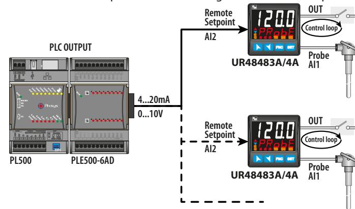
In this example the command setpoint is the value read on second analogue input AI2: on par. 55 *cPr.2* it is selected the input that determines the setpoint.
