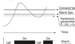
Upper deviation alarm value of alarm setpoint less than "0" and hysteresis value greater than "0" (Par.128  $R_{L.IH} > 0$ ).
