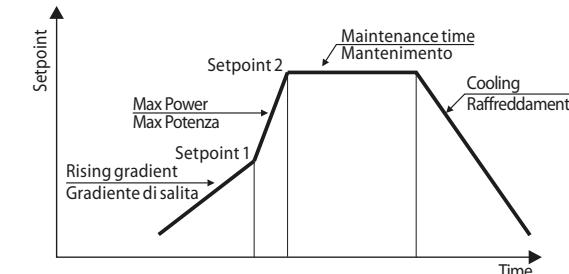
Cycle starts at each activation of the controller, or via digital input if it is enabled for this type of functioning (parameters 231, 239, 247, 255 set as *5E./5E.* or *RuN*).
