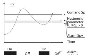
Lower deviation alarm value of alarm setpoint greater than "0" and hysteresis value greater than "0" (Par.128  $R_{L.IH} > 0$ ).
