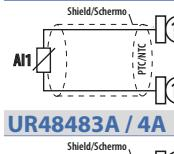
For thermoresistances NTC, PTC, PT500, PT1000 and linear potentiometers.
