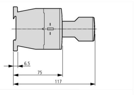
Contactor with auxiliary contact module
