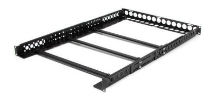
These 1U server-rack rails let you mount non-rackmount equipment such as desktop servers, networking equipment or KVM switches, into your 19" server rack without sacrificing 1U of rack space, like you would with a traditional shelf. The rack rails are also a great solution for mounting equipment with damaged rails or discontinued OEM equipment such as Dell<sup>™</sup>, IBM®, HP® or Apple servers that no longer have rack rails available.
