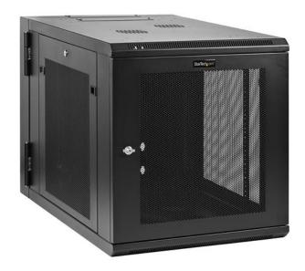
This 12U server or network rack cabinet lets you mount your EIA-310 compliant equipment to the wall, in a secure enclosure that has a hinged rear door for easy access to your equipment. The enclosure features adjustable mounting depth from 3 to 32 in. to provide a robust storage solution for your rackmount equipment.
