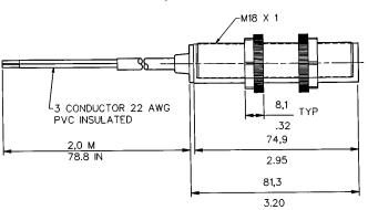
AC Connector Version Retroreflective/Diffuse Control, Thru scan Receiver
