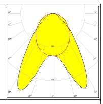
LED LM28xB Series **FWHM** Asymmetric 87 % Efficiency Peak intensity 0.620 cd/lm
