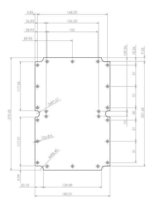
Dashed line shows outline of the mounting boss under PCB board Recommended mounting holes diameter ø3,5mm
