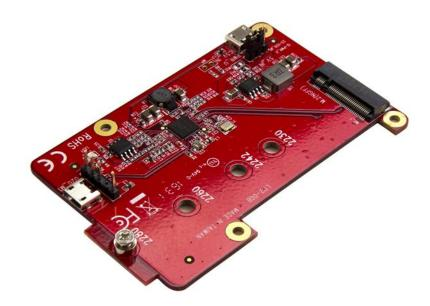
Increase the data storage capacity of your Raspberry Pi or other development board, by connecting it directly to an M.2 NGFF SATA SSD. Perfect for custom projects and applications, this USB to M.2 SATA converter supports all models of Raspberry Pi as well as other development boards.
