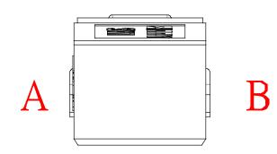
Marking will be random on side A or side B Markings are either by printing or molding Appearance according to dimensions drawing.
