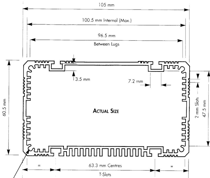
Suitable for No 6 x  $\frac{3}{8}$ " Pan Head Pozzi AB Screw
