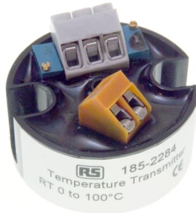
The 300TX is a 4-20mA temperature transmitter which can be housed in a probe terminal head suitable for a DIN standard block. With ranges for thermocouple and Pt100 sensors, the units offer an exceptionally wide range of span adjustment which reduces the need for stockholding different temperature ranges.
