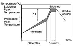
[Allowable Flow Soldering Temperature and Time]
