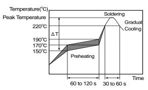
[Allowable Reflow Soldering Temperature and Time]
